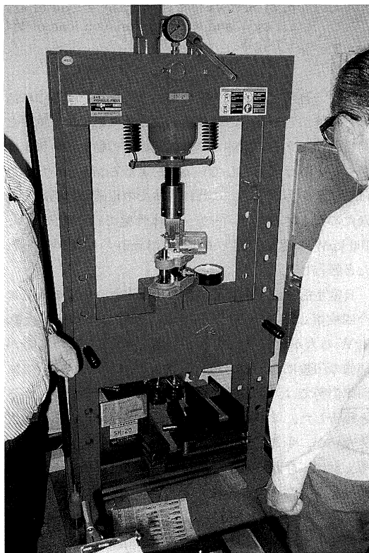
Fig. 3. Photo of the machine for three-point bending test.
